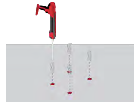
Figure 4 - Inject the resin.
