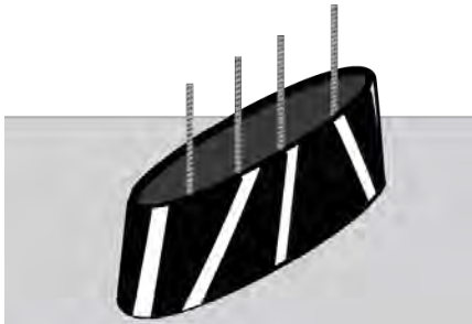
Figure 5 - Install the anchors. To ensure that the threaded rod is correctly anchored, it should be rotated while being inserted into the hole (full of resin) so that it is covered completely with resin. Once the resin is dry, tighten the first nuts with the socket wrench.
