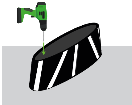
Figure 1 - Place a planter and mark the holes.
