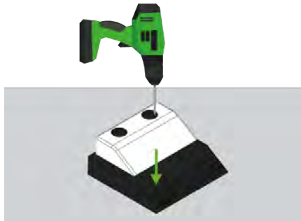
Figure 1 - Place the modules and mark the holes.
