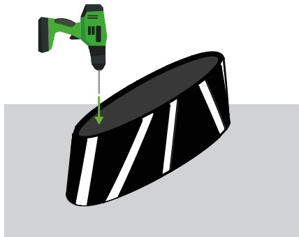
Figure 1 - Place the planter and mark the holes.
