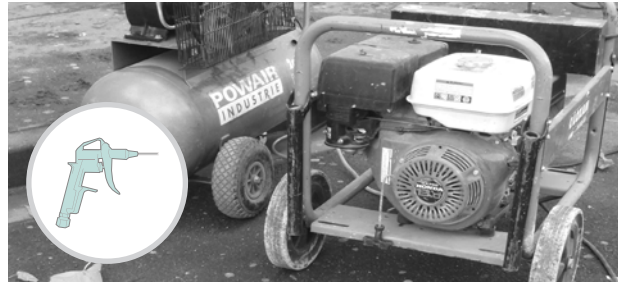
2. AIR COMPRESSOR TO REMOVE THE DUST THAT OCCUPIES THE HOLES AND A VACUUM TO AVOID THE DISPERSION OF THE DUST.
