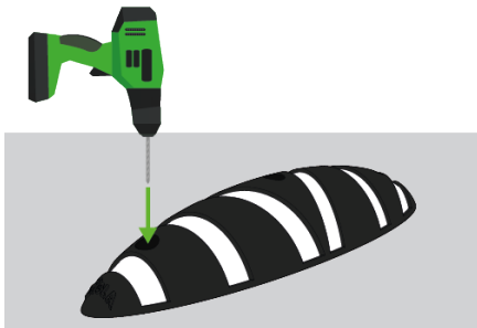
Figure 1 - Place the modules and mark the holes.
