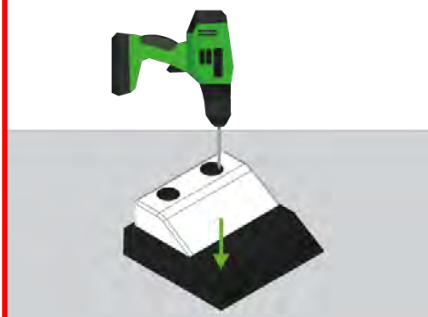
Figure 1 - Place the modules and mark the holes.
