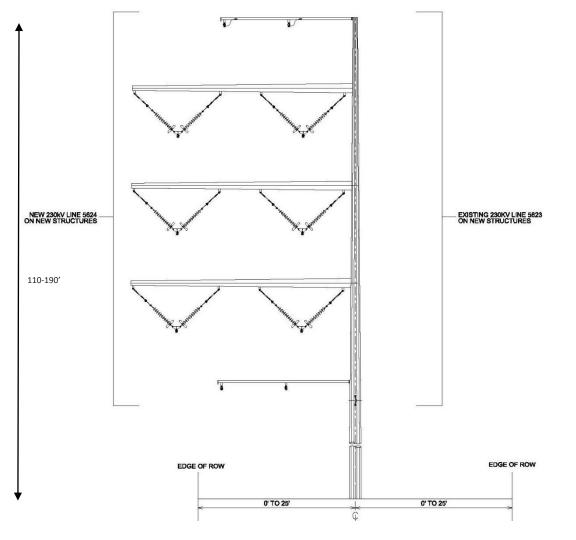
Rebuild 3.9 miles of the existing monopole single-circuit 230 kV transmission line to monopole double-circuit 230 kV.
