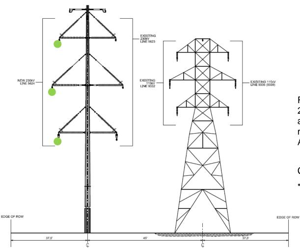
Re-energize the existing 115 kV to be 230 kV between Arapahoe Substation and Denver Terminal Substation for 2.0 miles (new structures needed at Arapahoe and South Substations).
