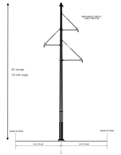
Rebuild 5.6 miles of existing 115 kV double-circuit lattice to 230 kV single-circuit monopole (tower for tower replacement).
