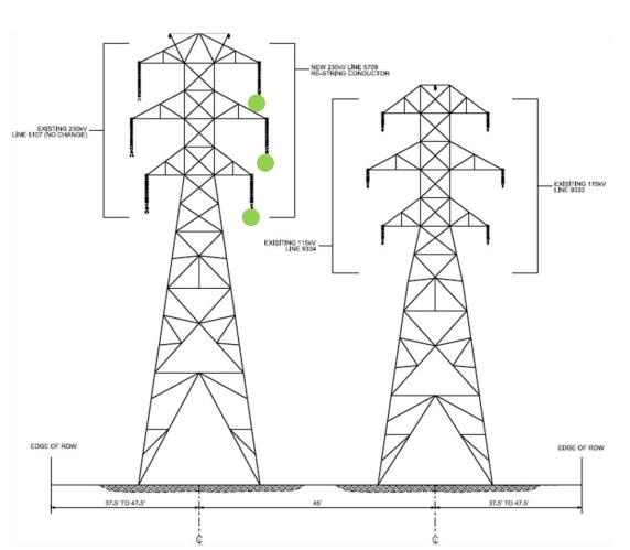
Reconductor 3.4 miles of existing 115 kV/230 kV, replacing the 115 kV circuit with 230 kV.
