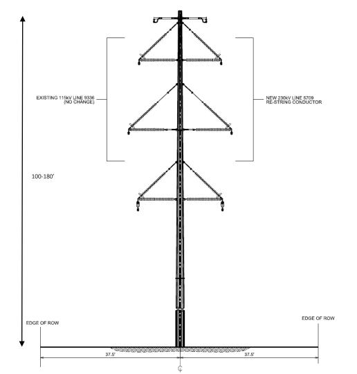
Remove four single-circuit 115 kV lattice structures for 0.5 mile; replace with four double-circuit monopole structures (230 kV on north side, 115 kV on south side).
