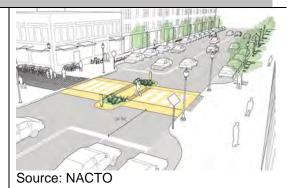
Reduce Corner Radii: The design radius of intersection corners determines the speed with which someone can take a turn at that intersection. Designing intersections with small corner radii can reduce motor vehicle speeds, increase driver awareness, shorten pedestrian crossings, provide additional space for improved ADA ramp design, and improve traffic control device visibility.
