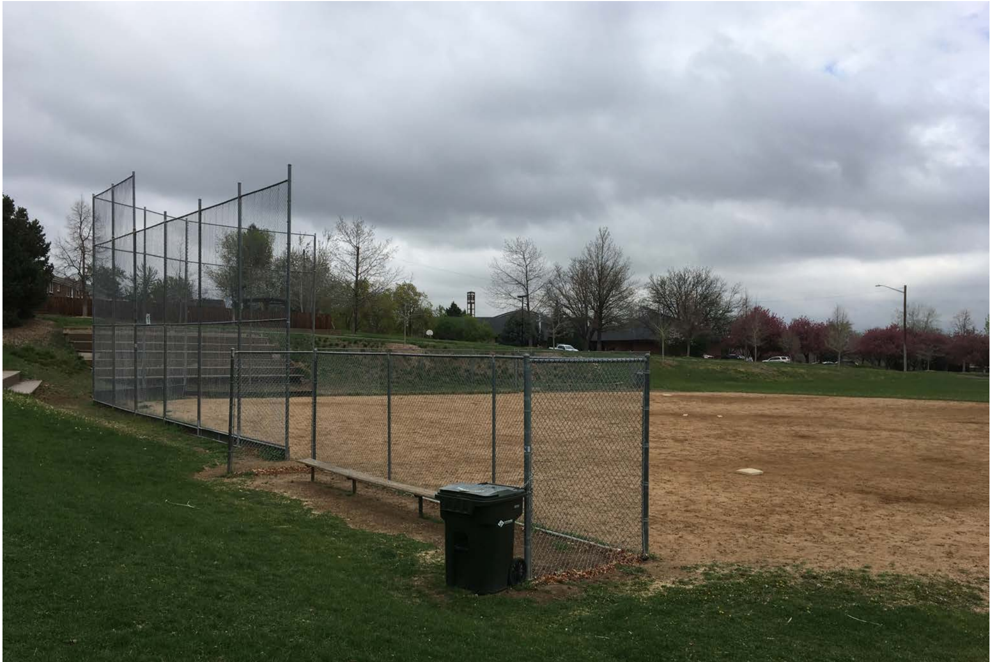
Image 9 - Northern ballfield - photo illustrates several deficiencies including: lack of an accessible route to field, bleachers and dugouts, and lack of accessible seating for players and spectators.
