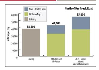
Of the additional 12,000 vpd associated with widening Broadway to six lanes, half of the new trips are projected to be Littleton trips, and the other half would be non-Littleton trips.
