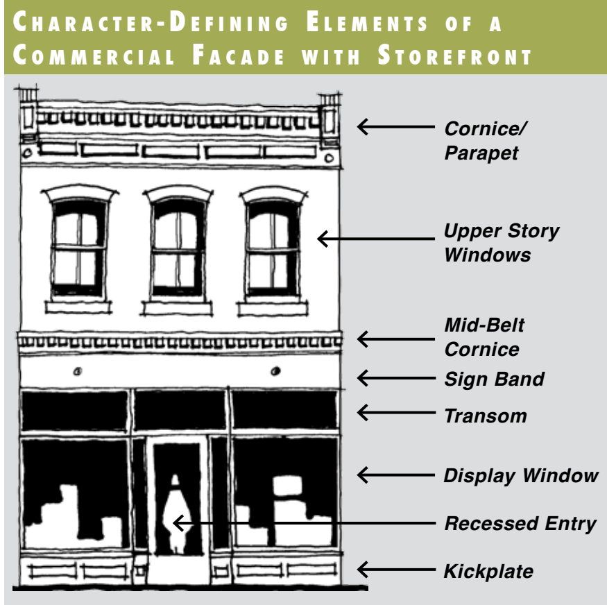
Diagram 1: Components of a commercial building facade with storefront.
