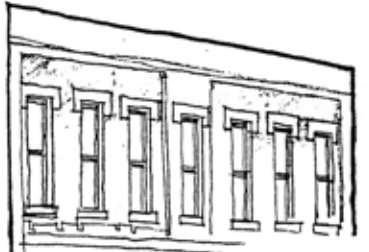
Existing building with missing cornice.
