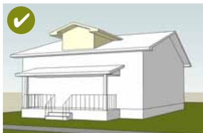
Small gable dormer Dormer addition is centered and located below the roof ridge.
