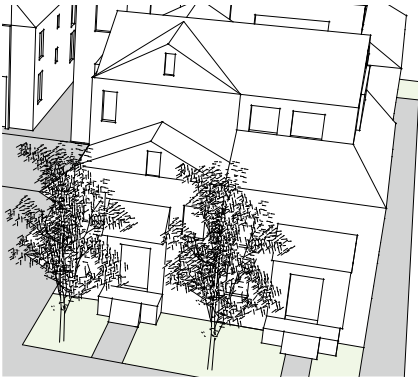
Design site and landscape improvements to promote energy efficiency where appropriate. In this example deciduous landscaping provides summer shading.
