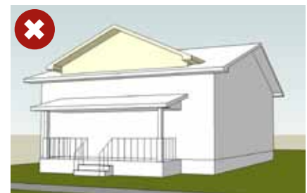
Full Gable Dormer Gable overwhelms the facade and alters the character.
