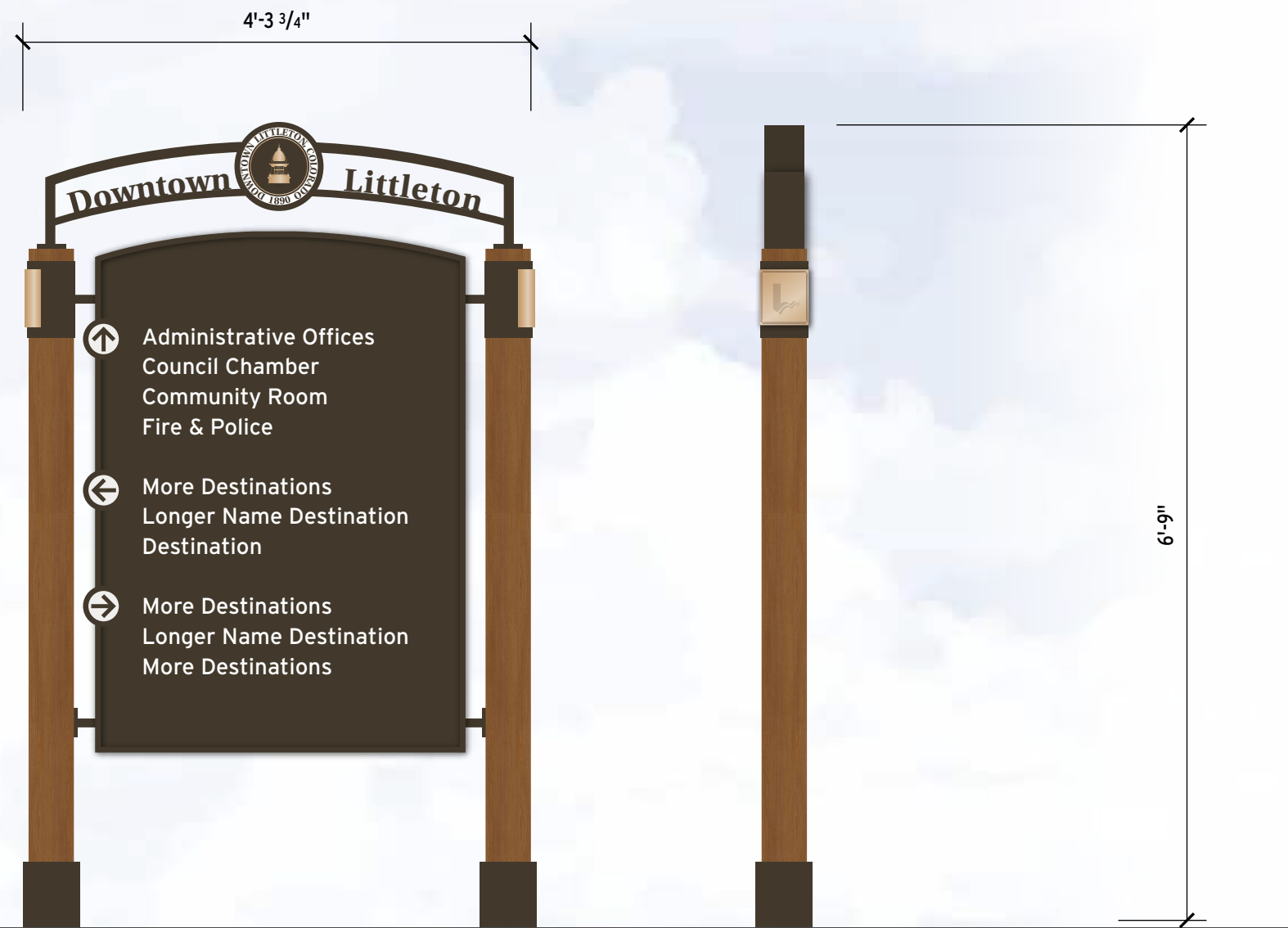
1 Pedestrian Wayfinding Sign - Front View Scale: 3/4" = 1'-0"
