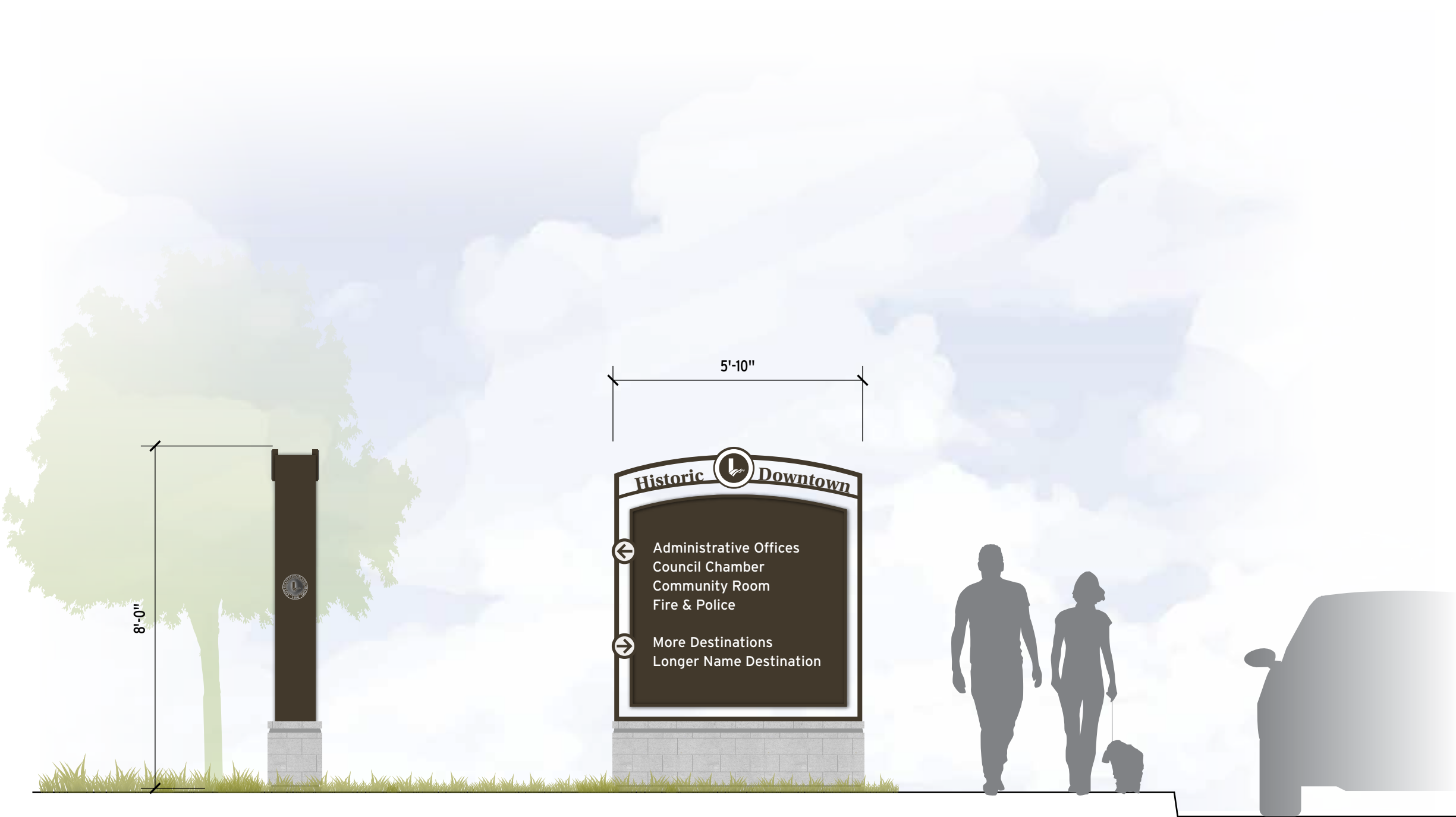
2 Vehicular Wayfinding Sign - Side View Scale: 3/8" = 1'-0"
