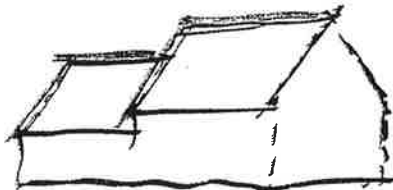
Roof stepped to break ridge line
