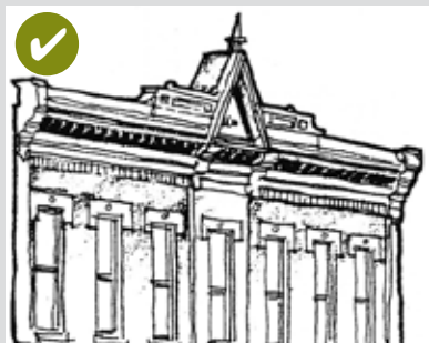
Reconstruct a missing cornice when historic evidence is available.
