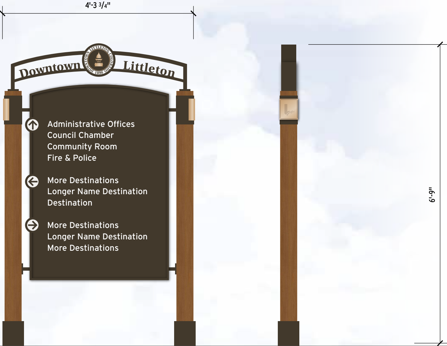
2 Pedestrian Wayfinding Sign - Side View - Scale: 3/4"= 1'-0"
