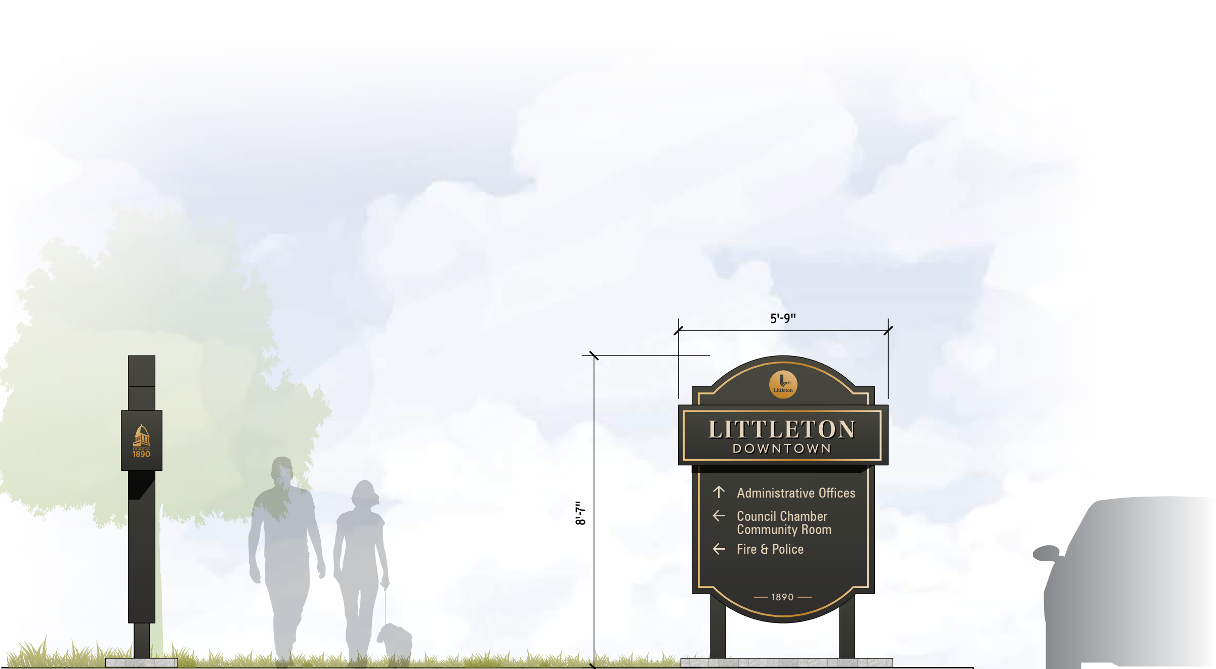
2 Vehicular Wayfinding Sign - Side View Scale: 3/8"= 1'-0"
