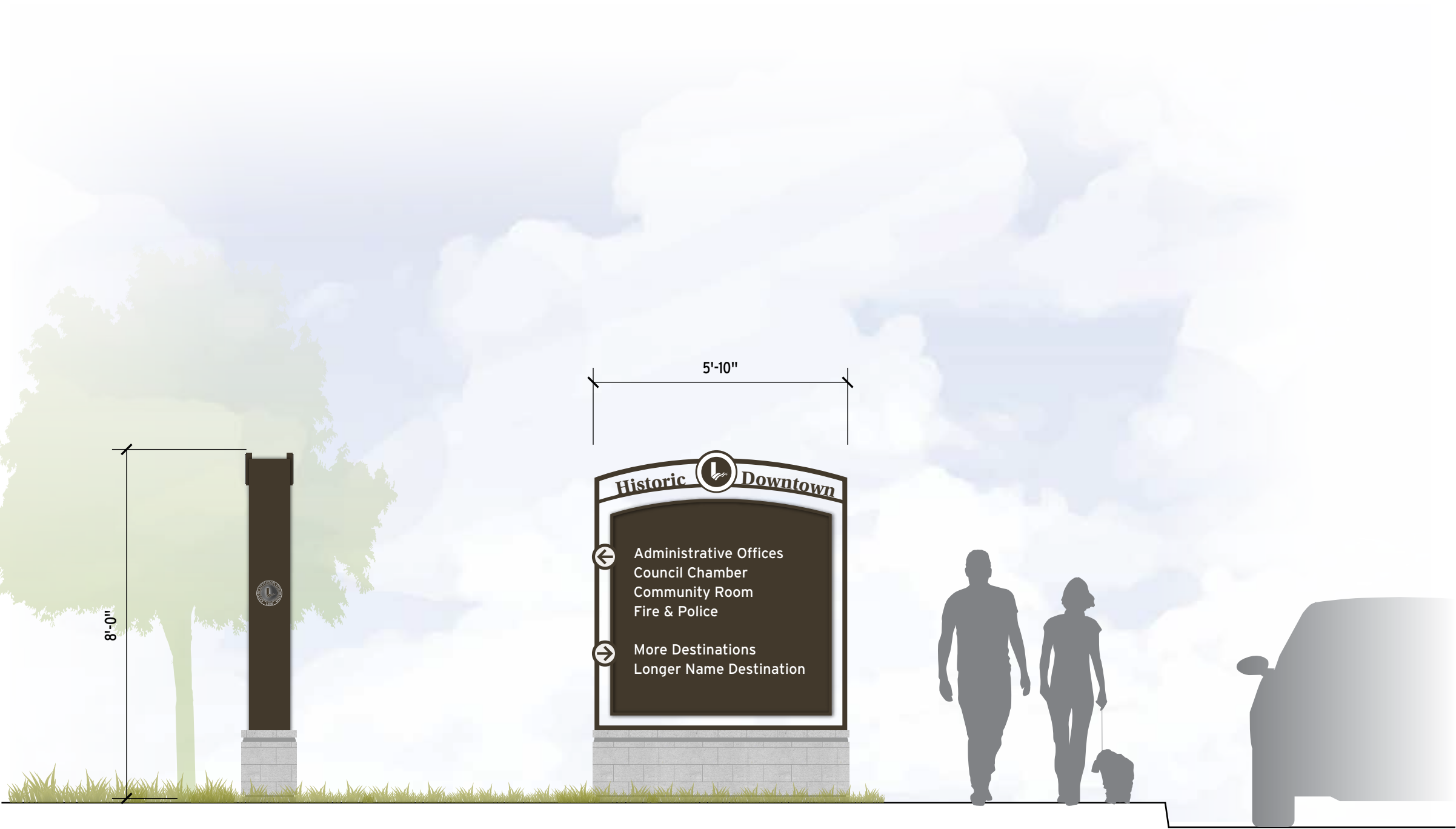
2 Vehicular Wayfinding Sign - Side View Scale: 3/8"= 1'-0"
