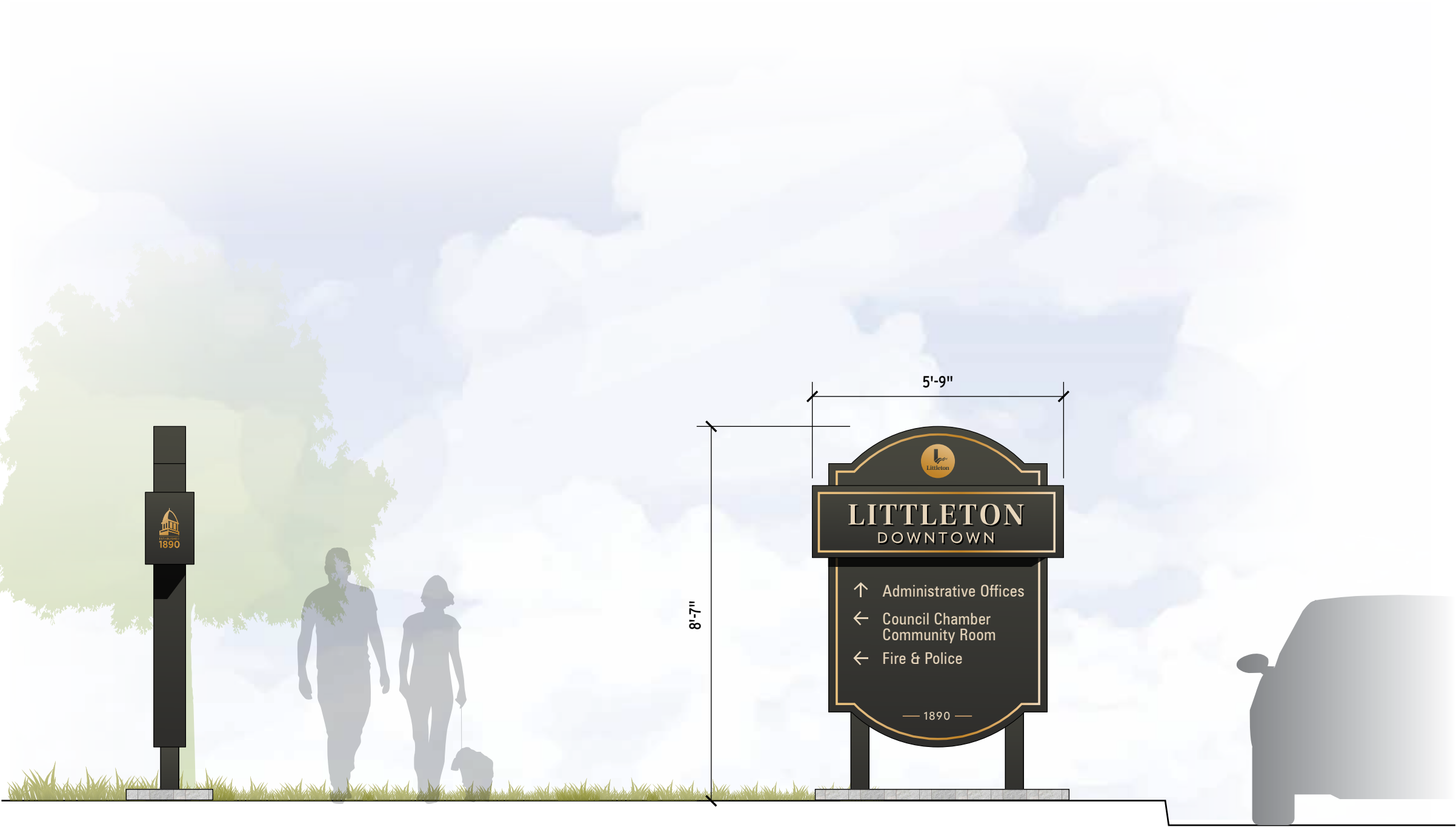
2 Vehicular Wayfinding Sign - Side View Scale: 3/8"= 1'-0"
