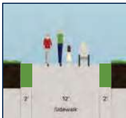
Figure 10. Alternative 3: Cross Section of Soft Surface Shared Use Path
