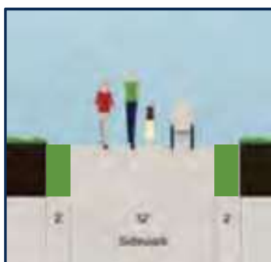
Figure 5. Alternative 1: Cross Section of Shared Use Path – East of Wolhurst Community
