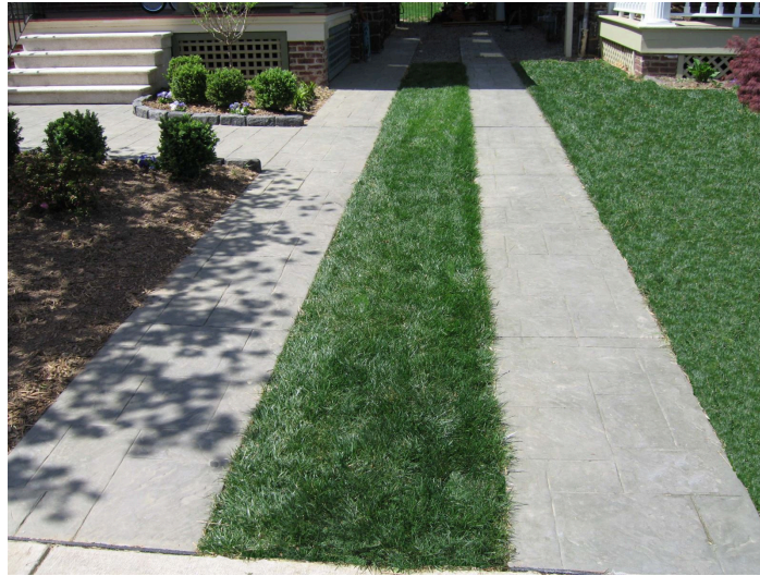
Figure 10-1-3.7.B.2 Wheel Strip Driveway Example
