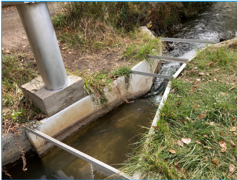
Figure 14: Parshall Flume located in the ditch just above its crossing of Big Dry Creek. Patented by Dr. Ralph L Parshall, a CSU professor in 1922, the invention made possible very accurate measurements of flowing water. Flumes of this type ended years of controversy over how much water was actually being used by ditch irrigators compared to their entitlement. Photo by author.
