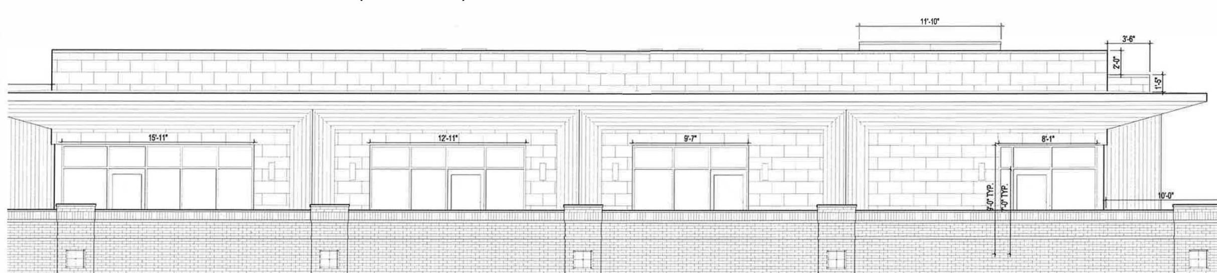
THIRD FLOOR DOORS, WINDOWS, BALCONY AND VISORS ALONG MAIN STREET (1/8" = 1'-0")
